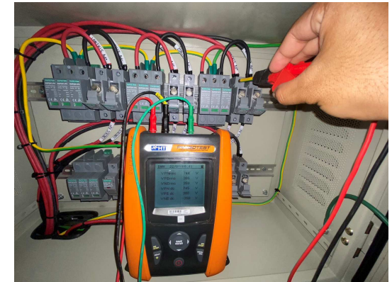
Earth protective continuity test and/or equipotential bonding
