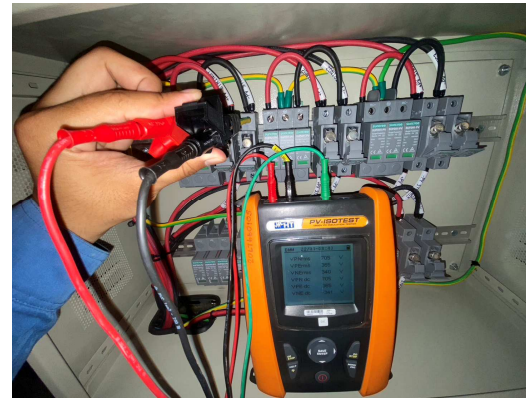
Earth protective continuity test and/or equipotential bonding
