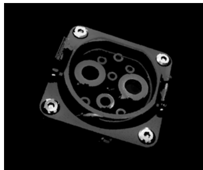
Car charging port
